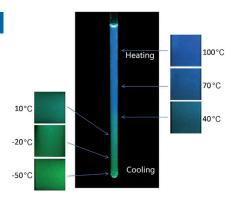
Feeling blue: The luminescence of a triarylboron compound has a high quantum yield (at least 0.64) over a wide temperature range (-50 to +100 °C) and changes from green to blue as the temperature is increased (see picture). The luminescence color was determined by the population of the two distinct excited-state conformations—a local excited state (high temperature) and a twisted intramolecular charge-transfer state (low temperature).
